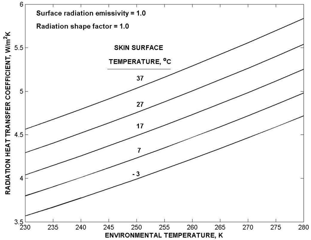
Figure 1: Radiation heat transfer coefficient
