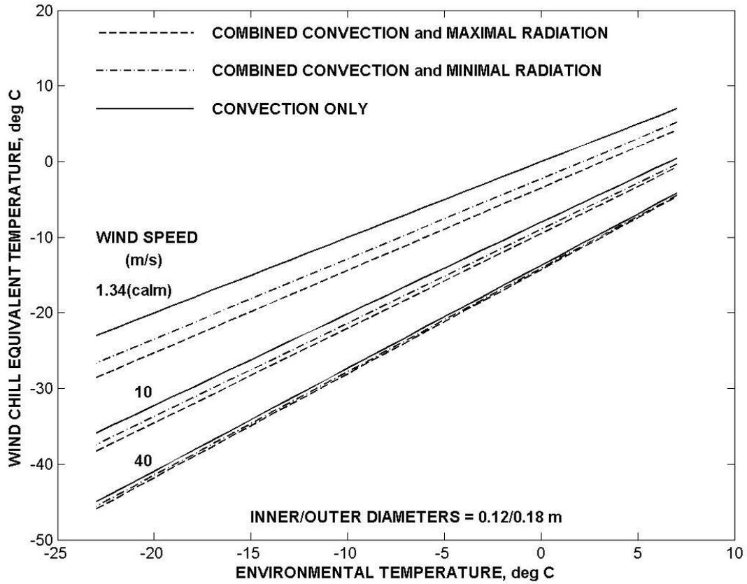
Figure 4: Wind chill equivalent temperatures calculated by wind-driven convection and by maximal and minimal combined effects of environmental radiation
