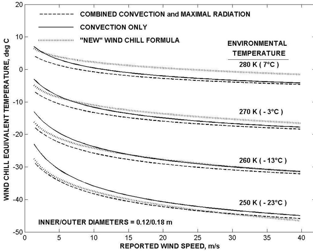
Figure 5: Wind chill equivalent temperatures calculated by wind-driven convection and by maximal combined convection-radiation compared to "new" wind chill formula (Environment Canada 2001)
