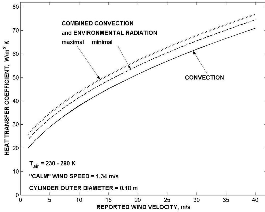
Figure 2: Wind-driven convection and upper and lower bounds of the combined convection-radiation heat transfer coefficients
