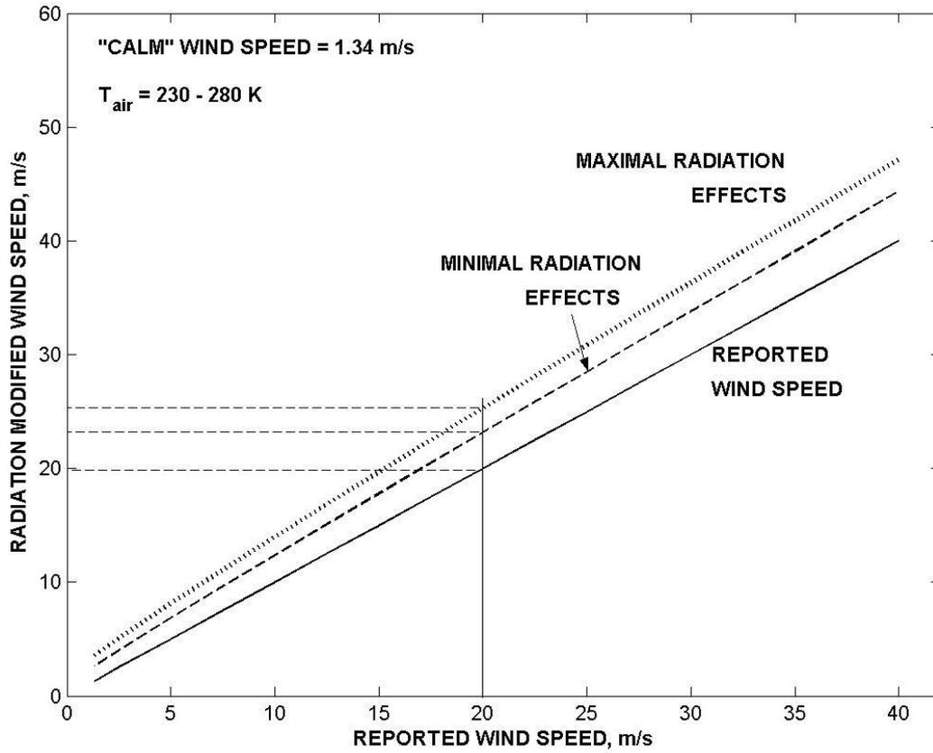
Figure 3: Upper and Lower bounds of the radiation-modified wind speeds
