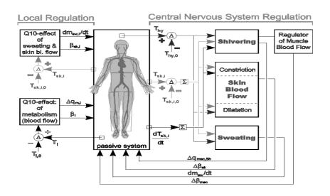
Figure 1 Schematic presentation of a physiological model of human thermoregulation (Fiala et al., 2001)
